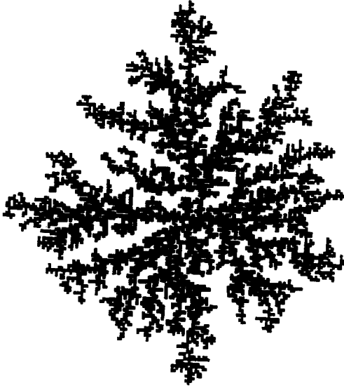
Figure 3. A cluster of 4630 sites generated using model II. In contrast to the patterns in a homogeneous medium (see reference [10]), the patterns generated in a random medium do not have an anisotropic structure for the same size clusters.
